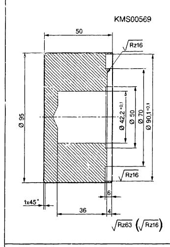
Thrust piece for supporting armature on undercutting saw/ for pulling off intermediate bearing:
